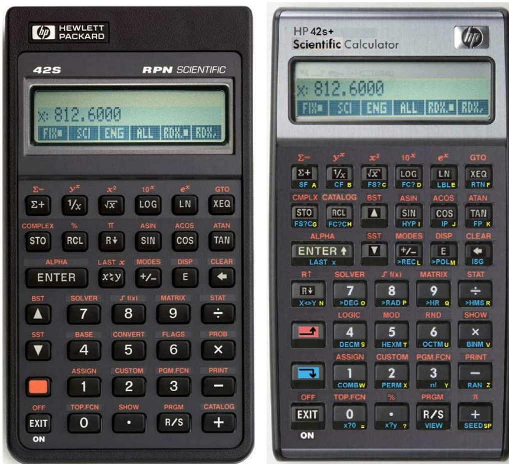
Fig. 7 - The original HP42S (left) and a proposed “HP42S+” (right) ported to the current HP17BII+ case.
