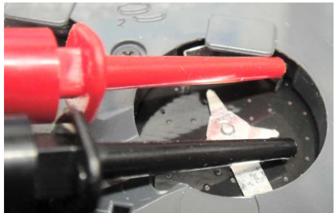
Fig. 7 – Typical CR 2032 cell connections.
