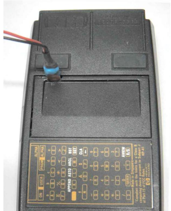
Fig. 5 – “Current probe” shown in place.
