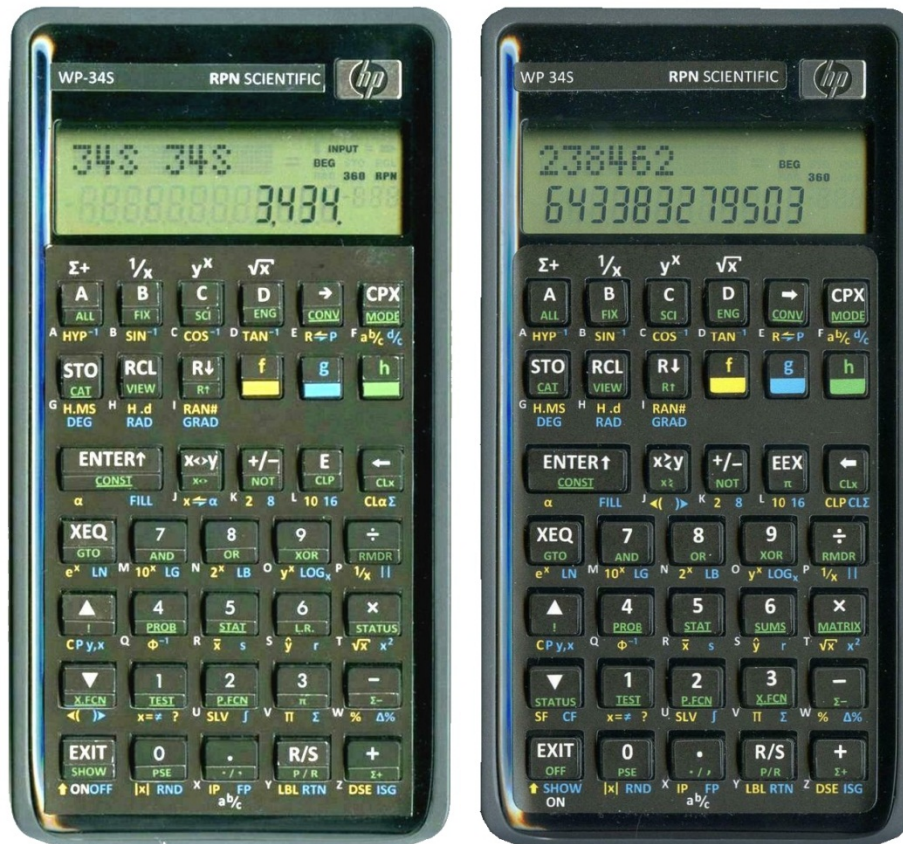
Fig. 1 - WP 34s Version 2 (left) and Version 3 (right). The Version-3 machine is in Double-Precision mode, displaying decimal places 16 through 33 of a popular irrational number.
