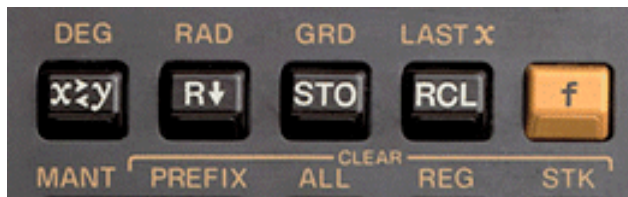
Fig. 13 – HP-31E STO and RCL related keys.
