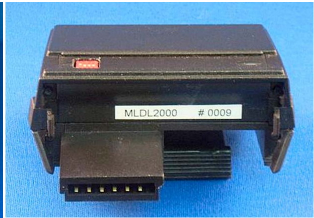
Fig. 4 - The modern MLDL2000, developed by Meindert Kuipers. This innocuous little device in the shell of a card reader provides 255 4k pages of ROM and 63 4k pages of user-programmable RAM. Enough storage capacity to virtually hold all ROM's ever developed for the HP-41.
