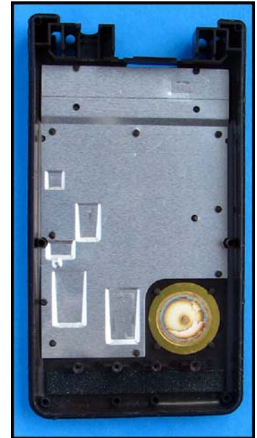
Fig. 23 - Shielding and piezo transducer.
