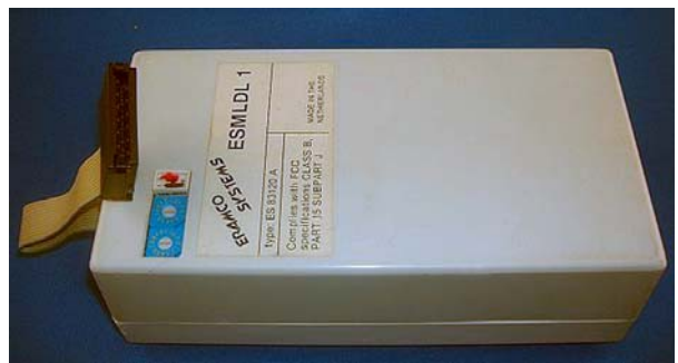
Fig. 2 - One of the first commercially available MLDL's was produced by the Dutch company Eramco. It provided 24k space for EPROMs and 8k of RAM into which the user could write MCODE using ERAMCO's operating system.
