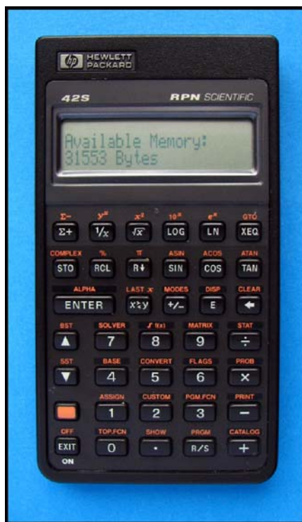
Fig. 34 - Upgraded memory HP42S with SIZE 025 and new keyboard flex PCB pressure pad.
