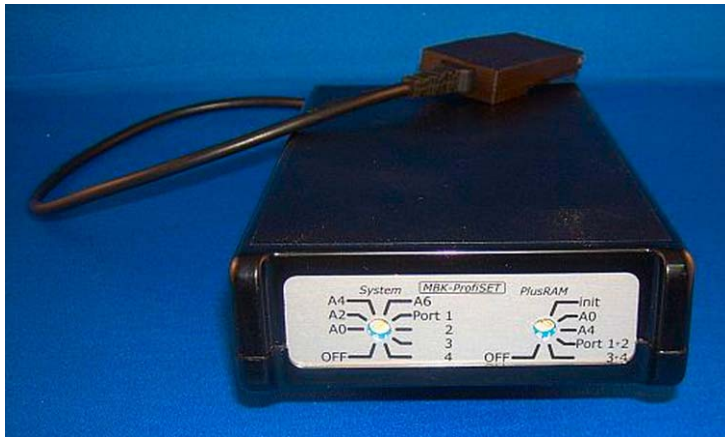
Fig. 3 - One of the most sophisticated MLDL's devices of its time, the ProfiSet was produced by the German Company MBK. It provided a full 32k of user-programmable RAM as well as 16k of ROM with one of the most comfortable operating systems to write MCODE as well as use the 32k RAM for extended program, ASCII file or data storage.
