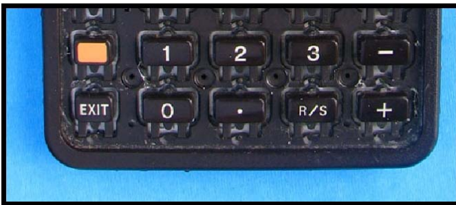
Fig. 17 – Four heat stakes under overlay.
