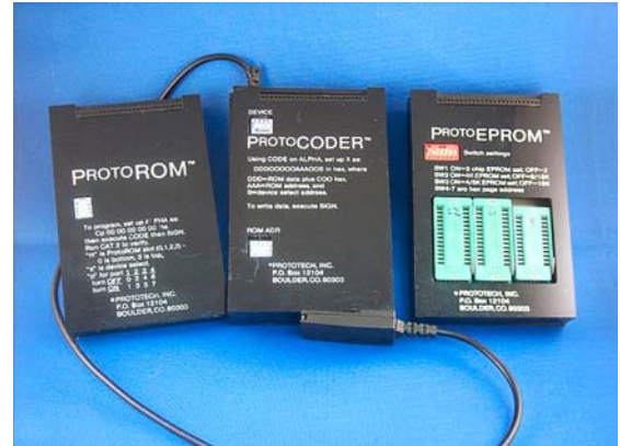
Fig. 1 - Nelson F Crowle was one of the earliest pioneers of MCODE development on the HP-41 and the developer of one of the first commercially available MLDLs. The above pictured ProtoROM and ProtoCoder each offers 4k of user-programmable RAM and 4k of ROM if used in combination with the ProtoEPROM.
