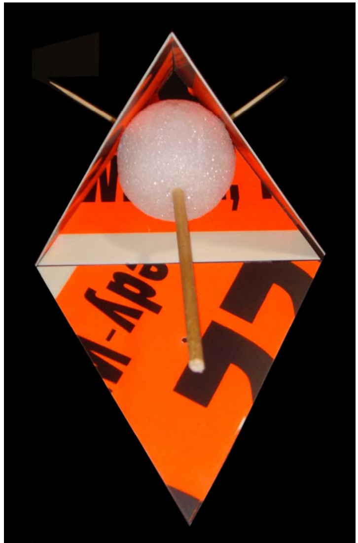
Fig. 4 – Styrofoam sphere in fixture with four holes to mark the equally spaced locations on the sphere.
