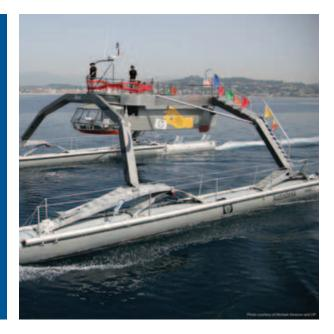
adjusts to the surface of the water. Its innovative superstructure is flexibly connected to specially designed pontoons to support the vessel and dramatically minimize stresses to structure, payload and crew. "Proteus does not pierce the waves; it dances with them," says Ugo Conti.
