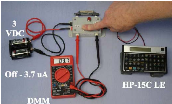
Fig. 3 – Off current being measured for HP-15C LE.
