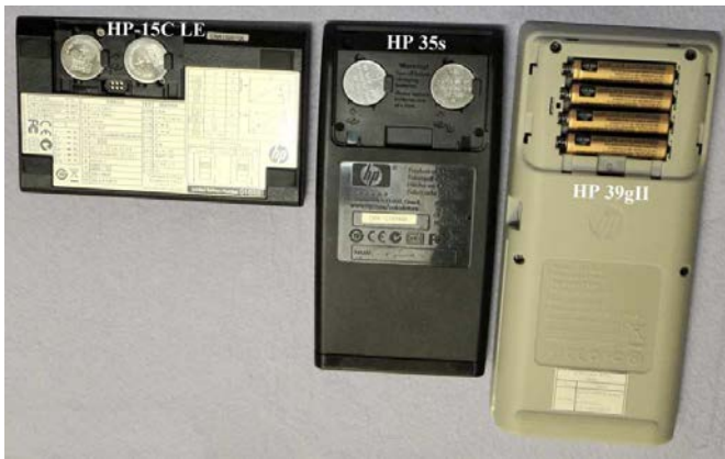
Fig. 14 – Scientific and Graphing Calculator cells.
