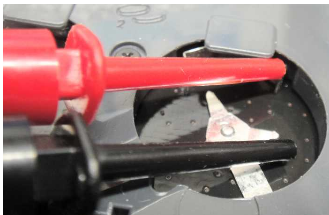
Fig. 7 – Typical CR 2032 cell connections.
