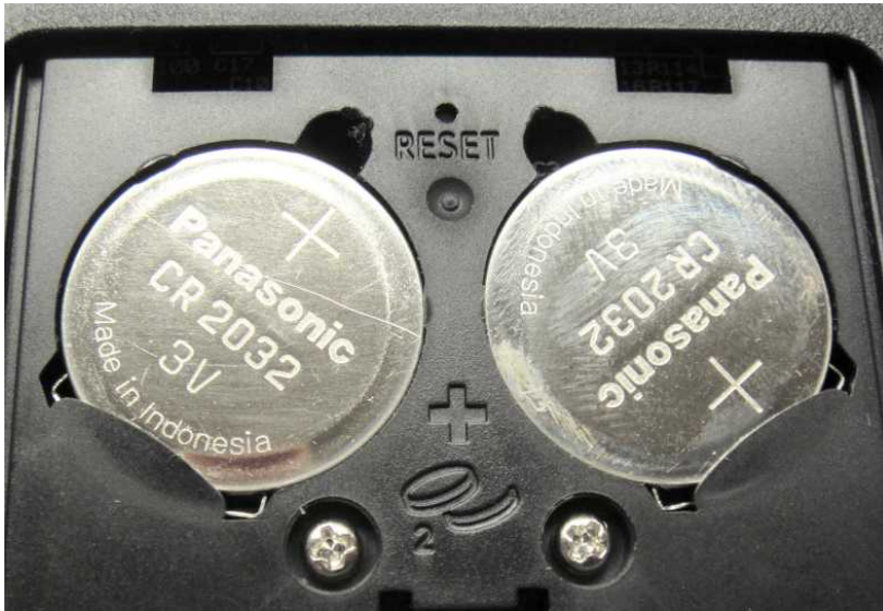
Fig. 6 – Coin cell holder with electrical connections “buried.”
