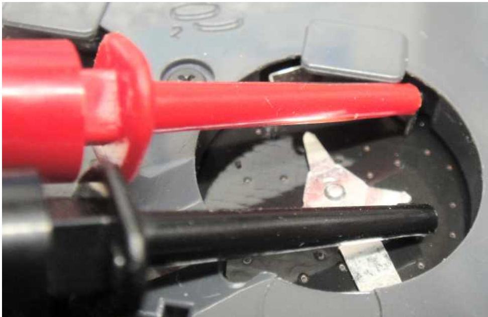
Fig. 8 – Miniature clips attached to the cell terminals; red positive, black negative.
