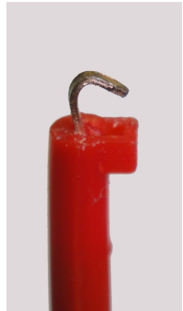
Fig. 8 – Miniature clips attached to the cell terminals; red positive, black negative.
