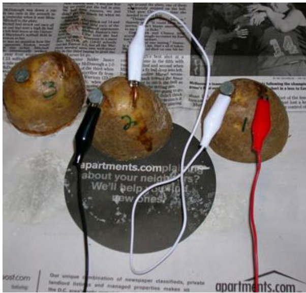
Photo 1: Two batteries in series
