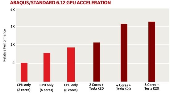
The effect of adding an NVIDIA Tesla K20 to a 2-, 4- and 8-core workstation shows a marked improvement in Abagus model processing performance.
