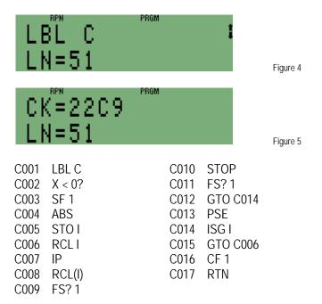
Answer: Run the program by pressing **1**.**01** (XEQ) **C** (ENTER). Since the input was positive, the HP 35s will pause and display each value stored in indirect registers 1 through 10. To have the HP 35s stop and display the value, key in the input as a negative number. Jake now has the program he wanted. NOTE: If you specify a range of bbb.eee which goes beyond the presently allocated indirect registers, this program will produce an error message.
